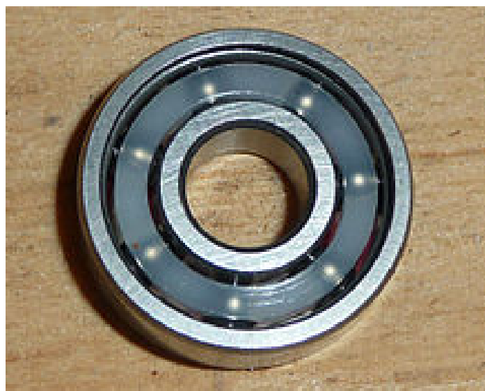
Fig. 11. A ball bearing for skateboard wheels with a plastic cage
